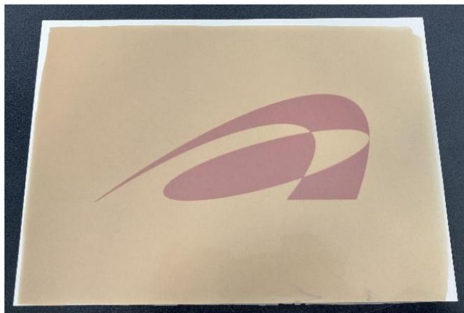
**Fig. 2.** Photograph of typical nonflammable and moisture-permeable UV protection films with approximately A4-paper size prepared from a clay mineral and SESC lignin (Li<sup>+</sup> montmorillonite: SESC lignin = 8: 2 w/w%).
