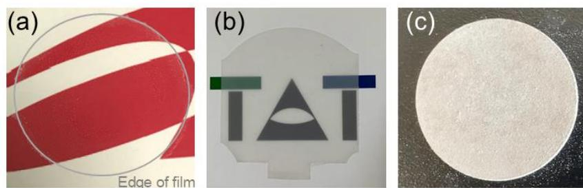
**Fig. 5.** Photographs of the transparent film consisting of hexyl modified SESC lignin obtained by solvent casting on PET substrate (a), PCL film containing 1 wt. % of hexyl modified SESC lignin (film thickness = ~0.3) (b), and pressed tablet of *m*-xylylene diisocyanate modified SESC lignin (XyDNCO).
